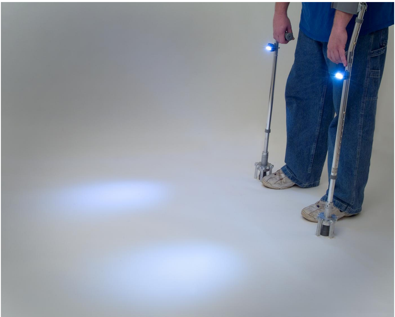
Fig. 11.66. Retractable Stability Mechanism Crutch with LED Navigation.
