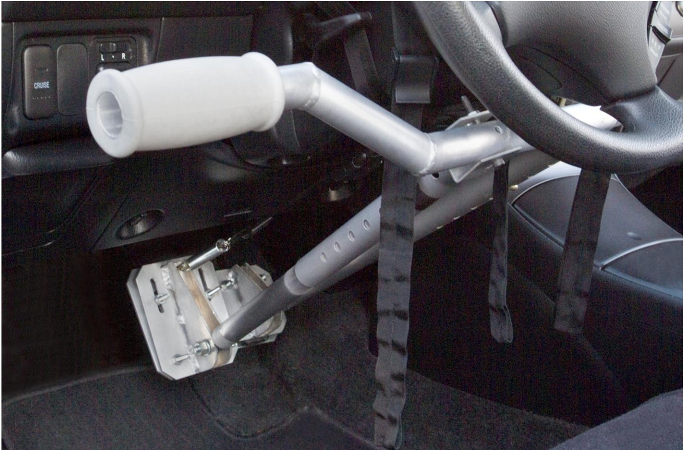
Fig. 11.31. Foot-Free Drive Assist Device Installed in an Automobile.
