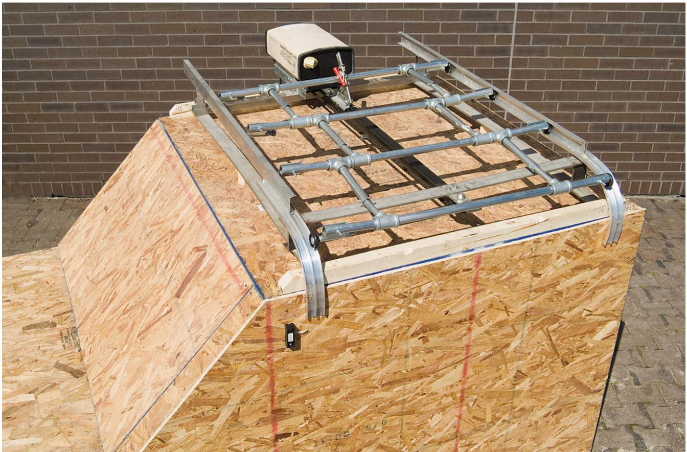
Fig. 11.56. Automatic Lowering and Raising Car Roof Rack System.
