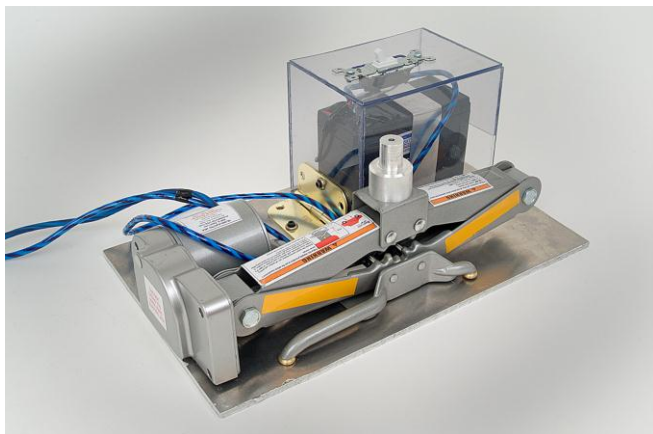
Fig. 11.25. Electric Jack Assembly.
