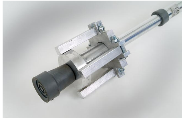
Fig. 11.64. Additional Leg Supports.
