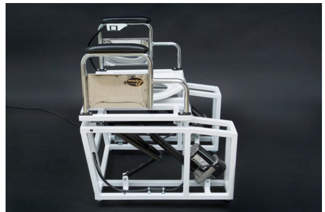
Fig. 11.3. Linear Actuators, Linkage Mechanism, and Armrests.
