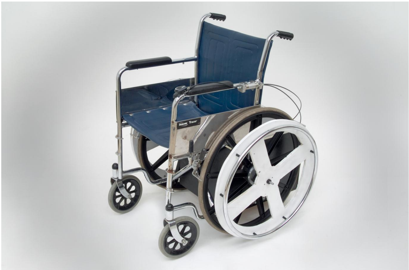
Fig. 11.42. Geared Manual Wheelchair with Variable Speeds.
