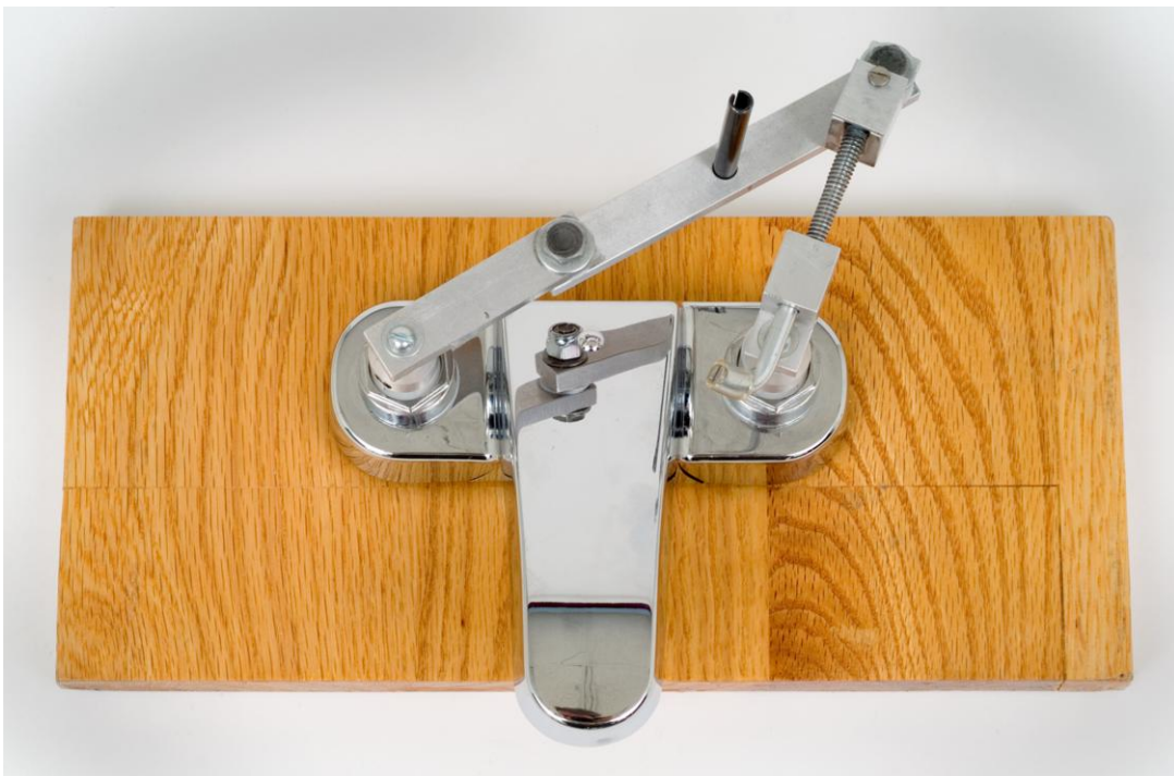
Fig. 11.87. Device Configuration When Faucet is Turned On.
