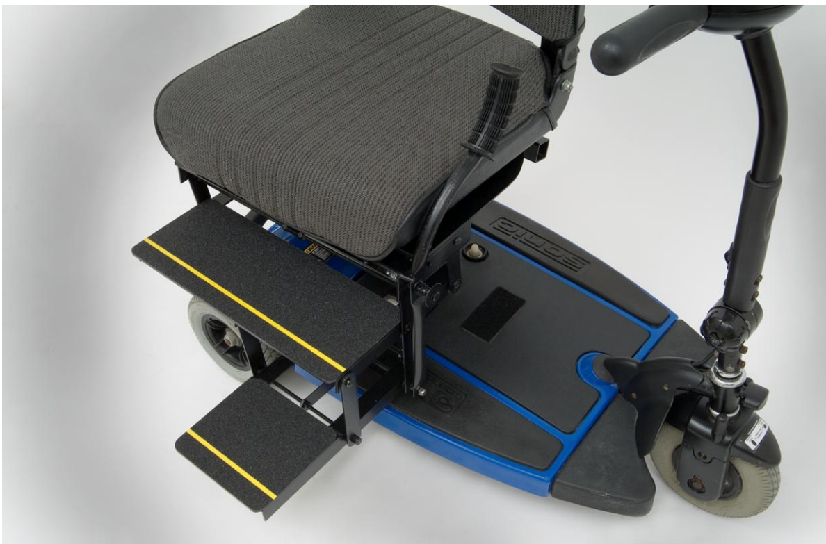
Fig. 11.72. Retractable Steps in Extended Position.
