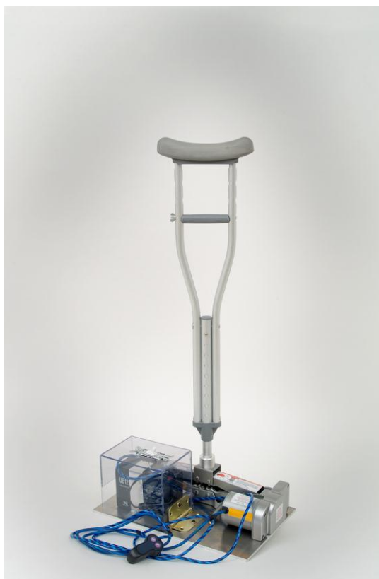
Fig. 11.27. Restroom Lift-Assist Device in Down Position.
