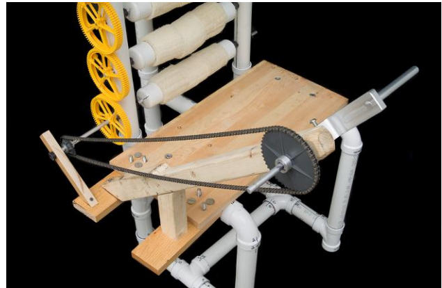
Fig. 11.28. Crank and Roller System.
