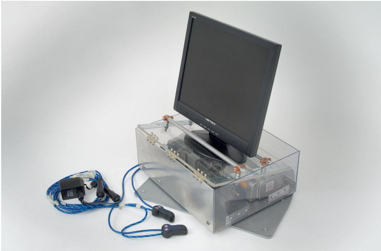
Fig. 11.7. Remote-Controlled Computer Monitor Stand.
