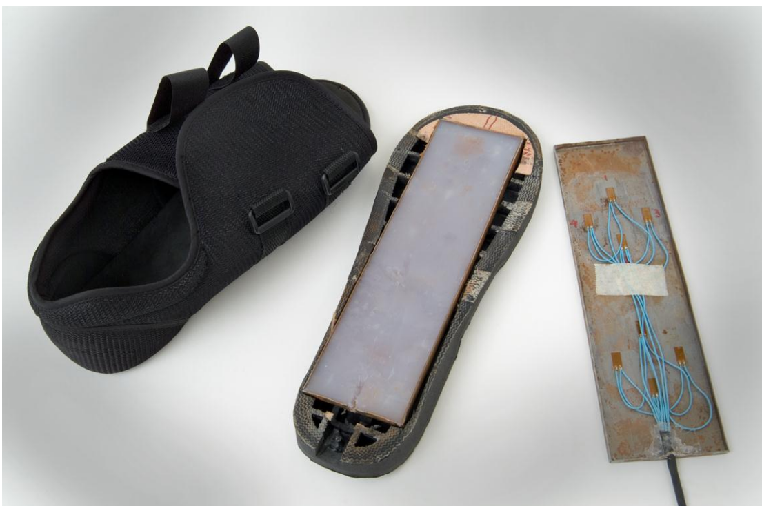
Fig. 11.35. Shoe and Strain Gauges.
